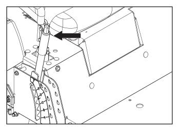
Mower deck lifting lever
